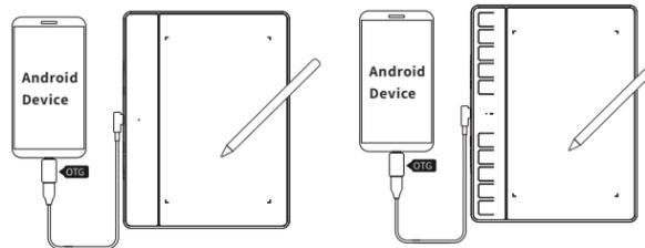
2. First, open an Android app that can support pen pressure, then rotate your pen tablet and Android device to vertical.
